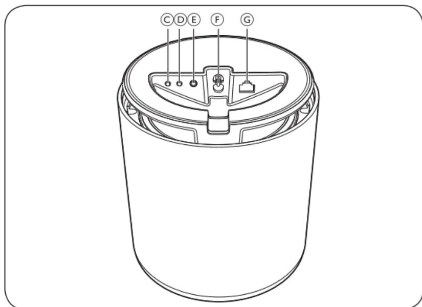
**EN** **C Standby button** Short press to put M5 in standby. Long press to turn M5 off. **D Configuration button** Short press to enter setup mode. When in setup mode, short press to cancel. **E Line in** Optical/Analogue mini-jack for connecting external audio sources. **F Power** Connect M5 to mains supply using only the enclosed mains cable. **G Ethernet** Ethernet socket for a wired network connection.
