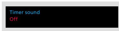
The Timer menu – the Off or On options decide whether sound is to be distributed to the TV speakers from a Timer play that you have made on your main room system.
