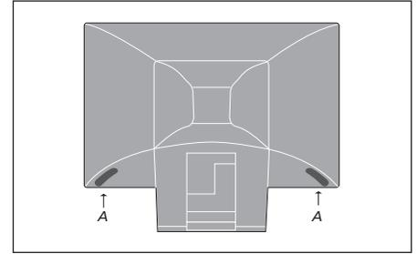
When lifting and moving the television, grip the recess (A) with one hand while steadying the television with the other hand at the top corner of the speaker. When lifting the television onto its stand (optional accessory) take care not to tilt the television while lowering it onto the guide pin on the stand.
