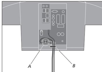
**IMPORTANT!** You must fasten the mains cord to the television using the cable brackets (A) and cable band (B). If this is not done, the cord can be tugged free of the socket.
