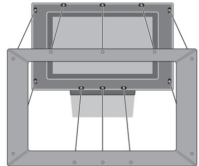
**To remove the speaker cover:** Gripping the top corners of the cover with your fingers, push inward on the screen with your thumbs until the speaker cover clicks free of the screen. Repeat the procedure with the lower corners of the cover, if necessary.
