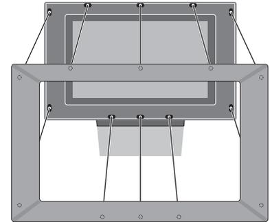
**Attaching the speaker cover:** Gripping the corners of the screen frame with your fingers, push it inward with your palms until the speaker cover clicks into place. Check all the contact points to ensure that the cover is securely in place.
