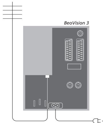
*If your television is equipped with the built-in system modulator, you will notice that the TV socket shown in the illustration is occupied, and that there is a second, unoccupied TV socket located just below a socket marked LINK. Connect your external TV aerial to this TV socket instead.*
