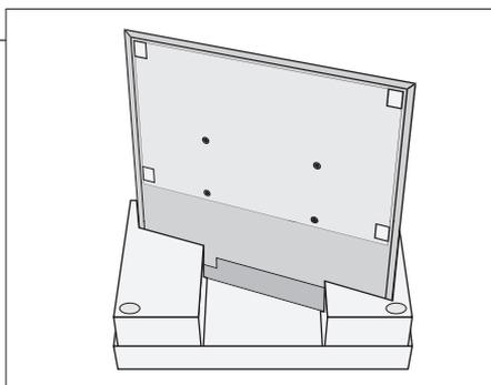
Three protection profiles have been enclosed with the TV. Use these when moving the TV to avoid scratching the frame.
