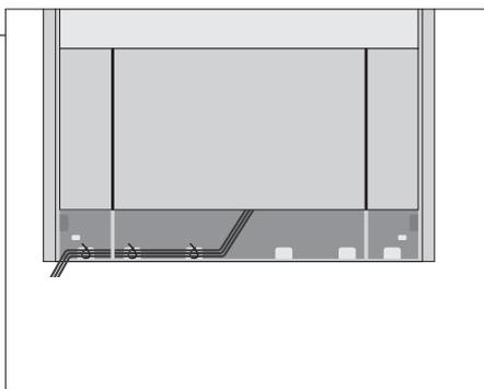
If you have a motorised stand, make sure that there is enough slack in the cables to allow the TV to turn to either side before you fasten the cables with cable strips to make a neat bundle.
