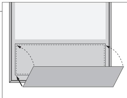
During cleaning it is recommended to remove the speaker cover. Avoid spraying liquid directly on the screen as this may damage the speakers, use a soft cloth instead. Carefully remove the speaker cover by supporting it in the side and at the bottom.
