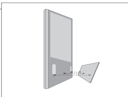
During cleaning it is recommended to remove the speaker cover. Avoid spraying liquid directly on the screen as this may damage the speakers, use a soft cloth instead. Carefully remove the speaker cover by supporting it in the side and at the bottom.
