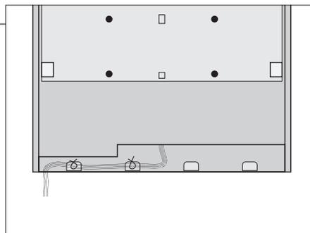
If you have a motorised stand, make sure that there is enough slack in the cables to allow the TV to turn to either side before you fasten the cables with cable strips to make a neat bundle.
