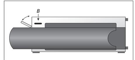
For access to the sockets for temporary connections, press the button (B) on the right side of the system and the door opens automatically. You can close the door manually.
