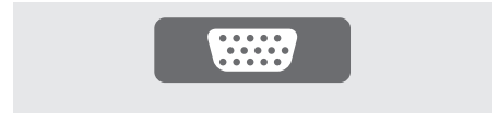
The PC IN socket on the back of BeoVision 4 for connection of a video signal from a PC.
