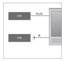
IR-transmitters: To operate non-Bang & Olufsen products with a Beo4/Beo6 remote control, attach a Bang & Olufsen IR-transmitter on your non-Bang & Olufsen product and then connect it to one of the sockets marked PUC on the connection panel. Attach the transmitter near the IR-receiver on the connected equipment to ensure remote control operation. Before attaching it, check that you can operate the equipment menus on the television screen using the Beo4/Beo6 remote control.
