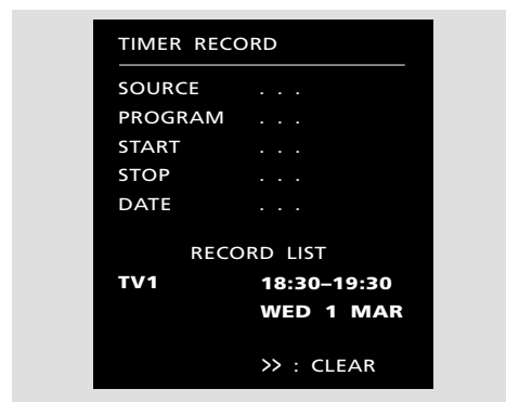
The Timer recording menu. A Timer recording is stored for TV program number 1, starting at half past six in the evening, on Wednesday the 1st of March.
