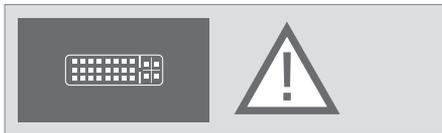
**IMPORTANT!** *If you wish to connect a computer to the television and use the television as a monitor, make sure that the television, the computer, and all equipment connected to the computer are all disconnected from the mains before you connect the computer and the television to each other.*
