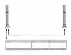
O SPEAKER LINK socket (using a *shielded* cable with 2-pin, 3-pin or 4-pin DIN speaker plugs)
