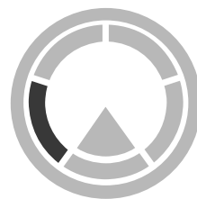
Figure 5.21: Press the curved line shown above to change the Beam Width to Wide with a Left Front direction.
