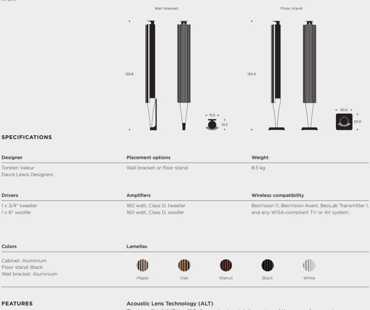
The benefit of ALT is a 180-degree horizontal dispersion of the upper frequencies, leading to uniform sound characteristics in the area in front of the loudspeaker allowing you to place yourself more freely and still get an optimal experience.
