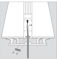
**Cable clamp:** For safety reasons the mains lead must be secured to the loudspeaker. To do so, place the cable cover with the cables behind the clamp, and tighten the two screws.
