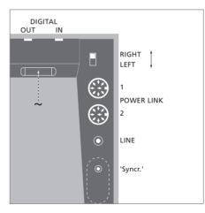
The 'Syncr. connection' is hidden beneath a small cover. To get access, just pry the cover off.
