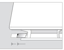
The moving microphone is used during the calibration. Make sure that there is always free space in front of the microphone.
