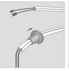
**Cable cover:** Place the mains lead and the signal cables inside the enclosed cable cover, and then use the special tool to seal the cover.
