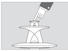
Press and hold the touch field for more than three seconds on the loudspeaker you wish to calibrate (while you are pressing, the indicator light quickly flashes red).
