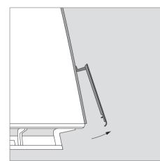
**Cover for socket panel:** To get access to the sockets and the RIGHT–LEFT switch, you will have to remove the cover. To do so, pull out the bottom edge of the cover, as illustrated above
