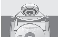
Press the LOAD button in the right-hand section of the operation panel to raise the clamp which holds the CD in place.
