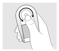
To operate the phone, you must use the wheel and the touch screen. Hold the phone and use your thumb to turn the wheel and to use the touch screen.
