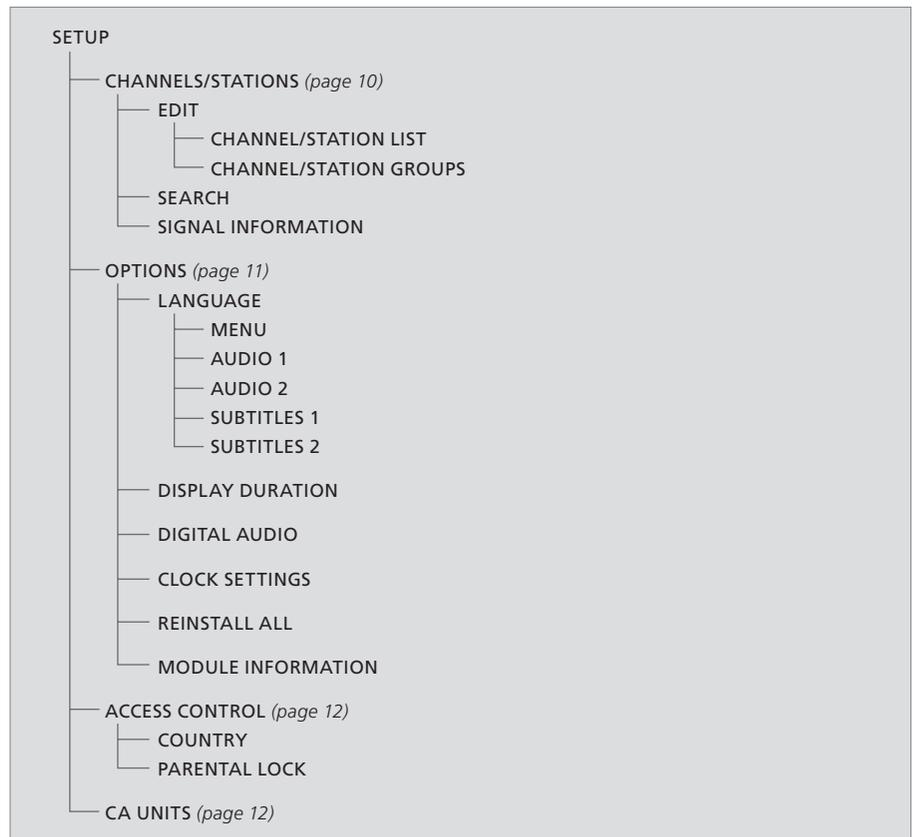
*Illustration of the structure of the Setup menu.
