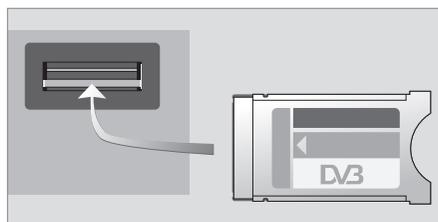
*The module must be inserted with the front facing up.*
