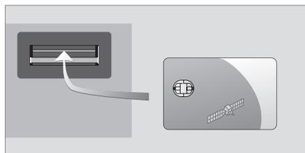
*Insert the Smart Card in the built-in CA-Module so the gold coloured chip faces upwards.*
